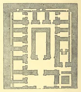
Fig. 78.—Crypts in the thickness of the walls, round the sanctuary at Denderah.
